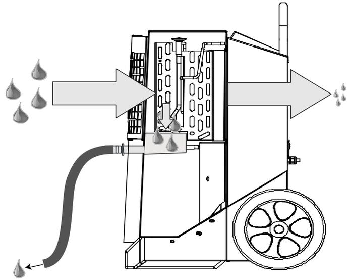
Due to the repeated air circulation through the dehumidifiers, the air humidity is continuously reduced whereby achieving rapid, but gentle drying.
