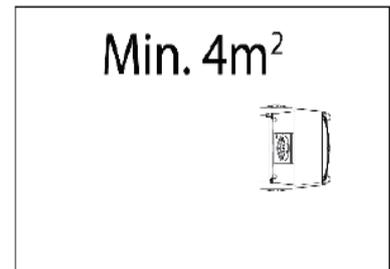
**Optimal operation:** Make sure that the room to be dehumidified is closed and the device is not placed near a heat source, such as e.g. a radiator.
