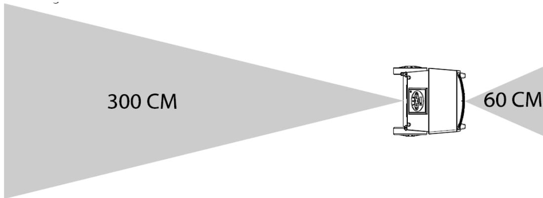
**Location requirements:** Since the appliances contain a flammable refrigerant, the following requirements for the location must be fulfilled.
